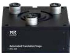
The ATS 204 is an automated translation stage that allows movement of the sample in X, Y, and Z via the Nanosurf stage control unit and accompanying software. Additionally, it can optionally contain a high-resolution 100- $\mu\text{m}$  Z-actuator with position sensor that is ideally suited for force spectroscopy measurements.
