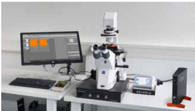
Adapters for many types of inverted microscopes are available. The motorized sample stage provides an easy way to combine inverted microscopy (bright field, phase contrast, and fluorescence) with AFM. It allows exact and reproducible position of microscope samples. In addition to the motorized sample stage shown above, a manual version is also available.
