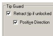
Select the behaviour of the system if the PLL circuit can no longer lock into the input frequency in order to prevent the tip from crashing. In this case the output is set to the maximum to force the z-feedback controller to retract the tip from the surface.
