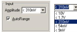
**Amplitude:** To set the sensitivity of the input amplifier circuit.
