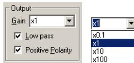
**Gain:** Sets the sensitivity of the output amplifier circuit (maximum output range is  $\pm 10V$ ).
