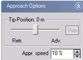
The slider defines the position of the tip during the approach. Normal position is in the center at 0 $\mu$ m. For surfaces with deep or high features close to the maximal z-scan range it could be better to set the tip position close to one side of the z-range. For surfaces with holes set the tip position closer to "Retracted". For surfaces with high small features set the tip position closer to "Advanced".
