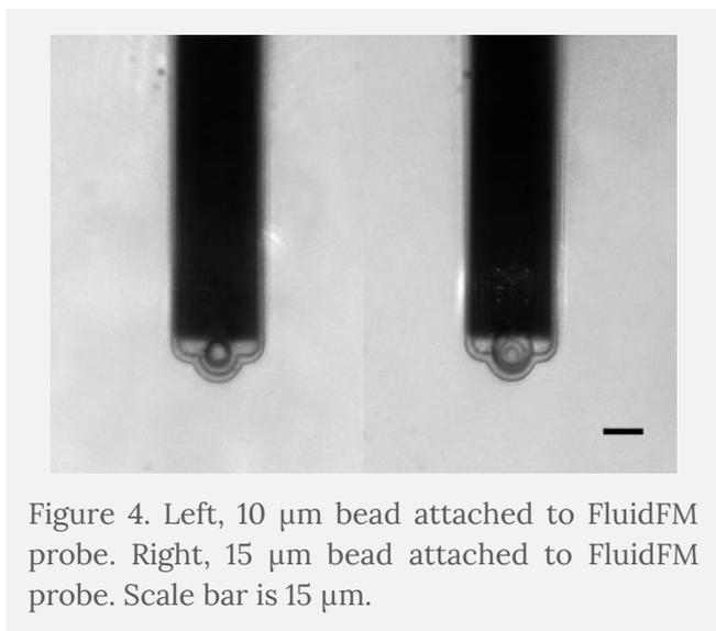
Figure 4. Left, 10 µm bead attached to FluidFM probe. Right, 15 µm bead attached to FluidFM probe. Scale bar is 15 µm.
