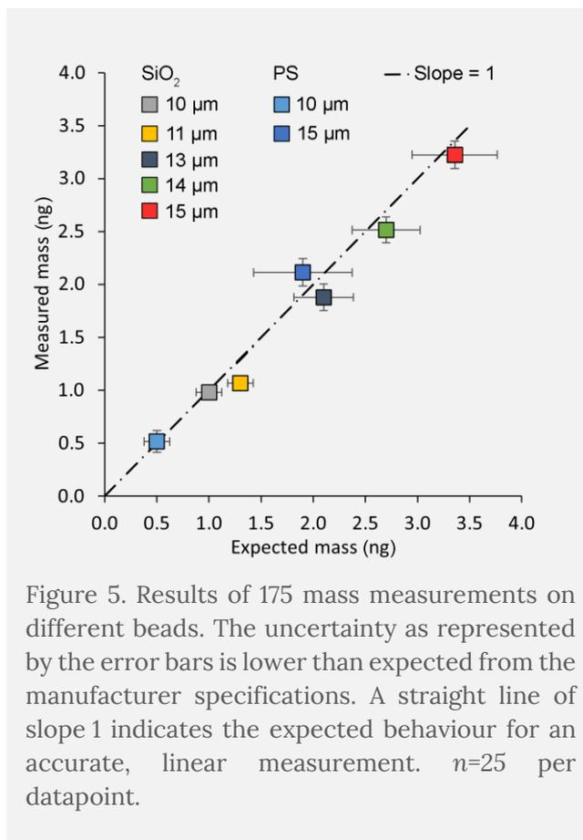
Figure 5. Results of 175 mass measurements on different beads. The uncertainty as represented by the error bars is lower than expected from the manufacturer specifications. A straight line of slope 1 indicates the expected behaviour for an accurate, linear measurement.  $n=25$  per datapoint.
