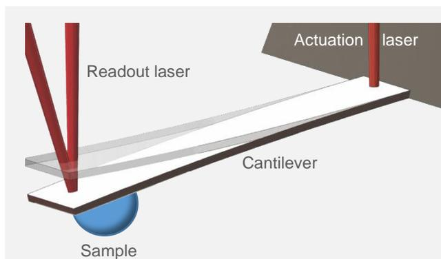
Figure 1. PicoBalance schematic. The mass of a sample is measured by determining the mass-induced shift in resonance frequency of an oscillating cantilever. Actuation and readout are done via near-infrared lasers.
