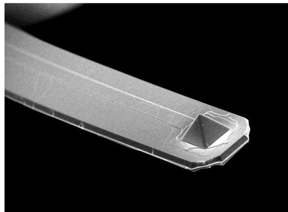
**Figure 3. Scanning electron micrograph of a VertiSense AFM cantilever.** The cantilever bears a tiny thermocouple element at the apex of the AFM cantilever tip. The material around the thermocouple is thoroughly chosen to prevent heat loss from the thermocouple into the cantilever material. Thus, precise temperature
