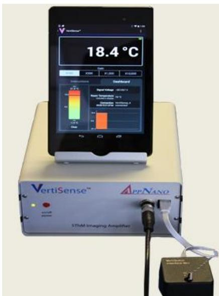
**Figure 2. The VertiSense Imaging Amplifier.** It connects to the VertiSense cantilever and the Nanosurf AFM controller. The Imaging amplifier is controlled via a tablet or smartphone application.
