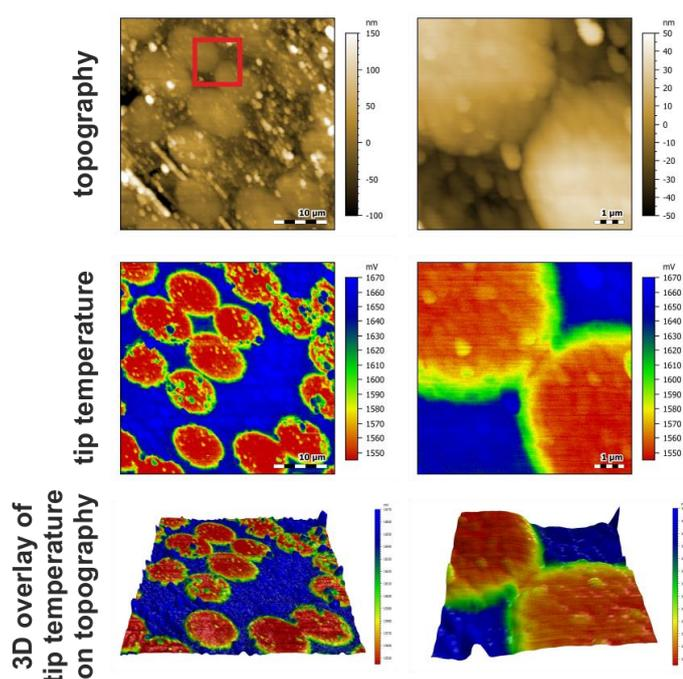
**Figure 1. AFM imaging and thermal analysis of polymer-embedded carbon fibers.** AFM topography (top), tip temperature (uncalibrated Imaging Amplifier output, middle) and tip temperature mapping to the 3D sample topography representation (bottom). Images in the left column show a 40 µm sample area, while the images in the right column were recorded inside the area indicated by the red square shown on the topography image in the left column.
