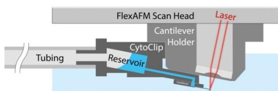
FluidFM probes have a closed channel connecting the cantilever opening to a fluid reservoir. A controller is used to vary back pressure to the reservoir to allow deposition parameterization. Force control is obtained through laser-based measurement of cantilever bending by the AFM that is an integral part of the FluidFM system.
