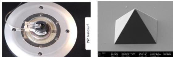
Left: Mounted hollow cantilever with tubing connected to the reservoir.
