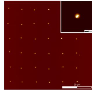
Air environment, 100 mbar back pressure, 50 ms contact time. Diameter:  $615 \pm 60 \text{ nm}$
