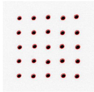
Air environment, 250 mbar back pressure, 1 s contact time. Diameter:  $4.83 \pm 0.17 \mu\text{m}$
